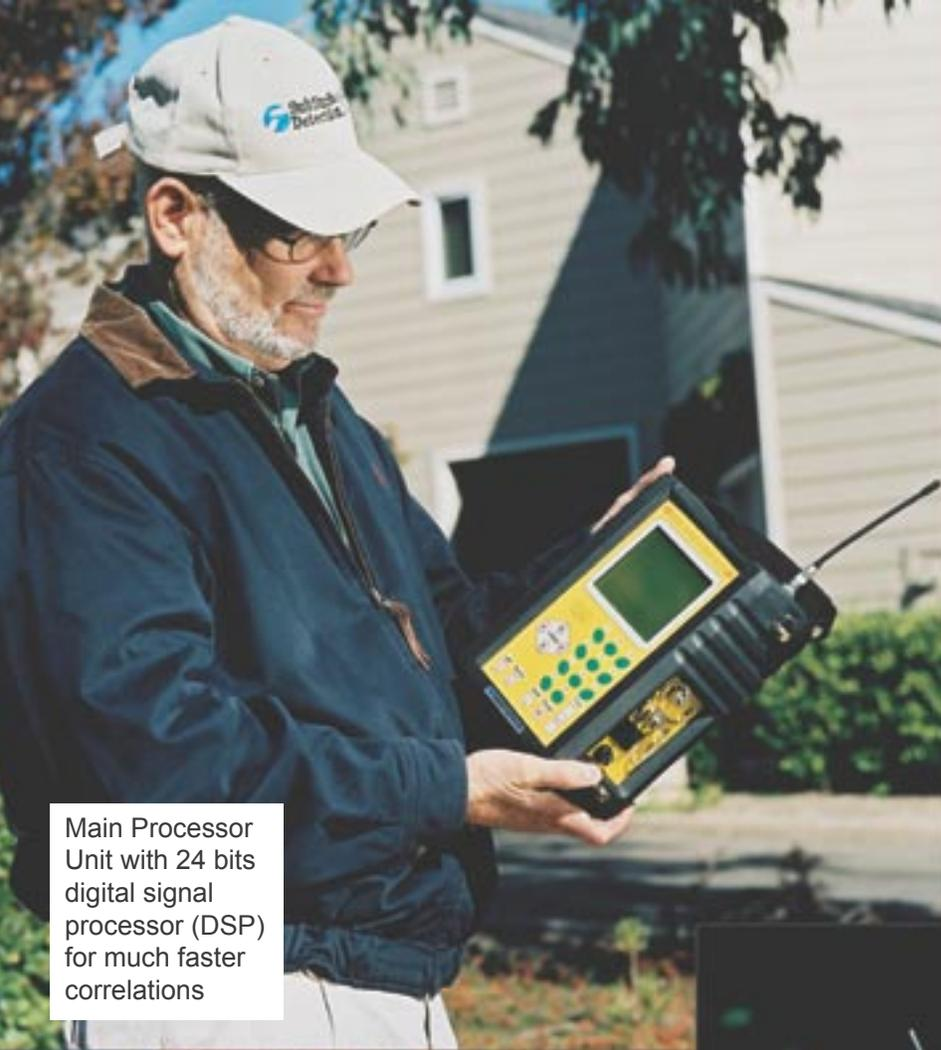
Main Processor Unit with 24 bits digital signal processor (DSP) for much faster correlations
