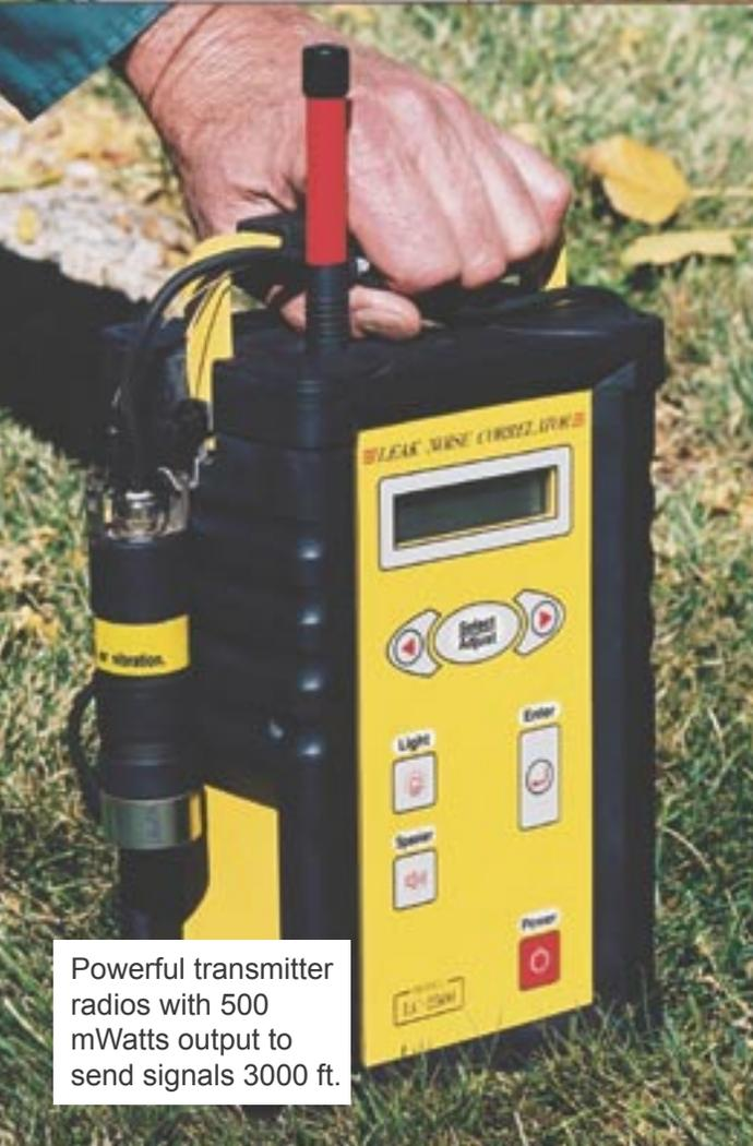
Powerful transmitter radios with 500 mWatts output to send signals 3000 ft.
