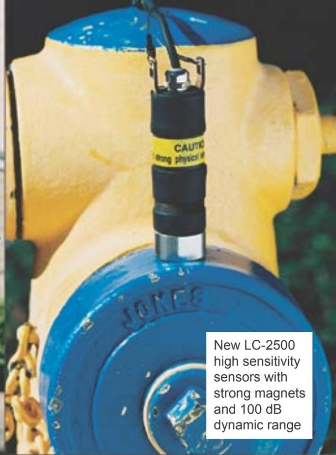
New LC-2500 high sensitivity sensors with strong magnets and 100 dB dynamic range
